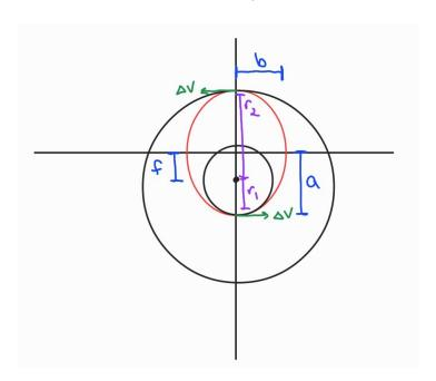
Plugging in  $r_1 = 21000$  and  $r_2 = 42300$  into  $2a = r_1 + r_2$ , we find that a = 31650. Then, plugging in a = 31650 and  $r_1 = 21000$  into  $f = a - r_1$ , we find that f = 10650. Then, subbing
