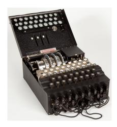
Essentially, the Enigma machine was an elaborate keyboard with sets of dials. A configuration of the dials would determine a method for scrambling the plaintext letters, in such a way that each successive plaintext letter is encrypted differently from the last. When a plaintext letter was typed into the keyboard, the corresponding ciphertext letter would light up elsewhere on the machine.
